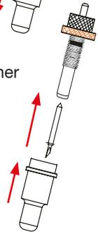
3. Adjust the amount of exposed (visible) blade tip to a suitable length by rotating ② the "Adjustment depth knob" and then tighten the lock ③.
