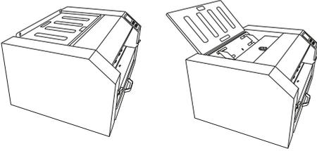
When deciding where to position, the Intec LC600, open the Media support tray (TOP) ready to accept media to be cut.
