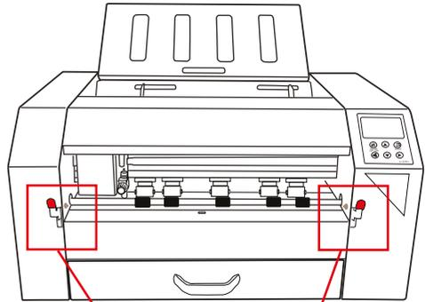
2. Open the Dual Drip Lever clamps to remove the Dual Grip Roller. In order to release the Dual Grip Lever, press in the ball catch ②. (You may find it easier to use the end of a pen to do this).
