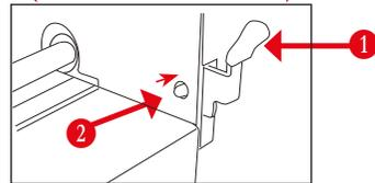
3. Once the Ball catch has been depressed, you can press the red catch down, to open the Dual Grip Roller clamps.
