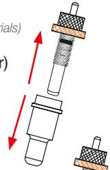
2. Insert the blade into the inner blade holder. Then replace the outer cover of the blade holder;
