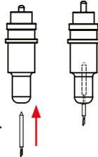
2. Adjust the amount of exposed (visible) blade tip to a suitable length by rotating ② the "Adjustment depth knob" and then tighten the lock ③.
