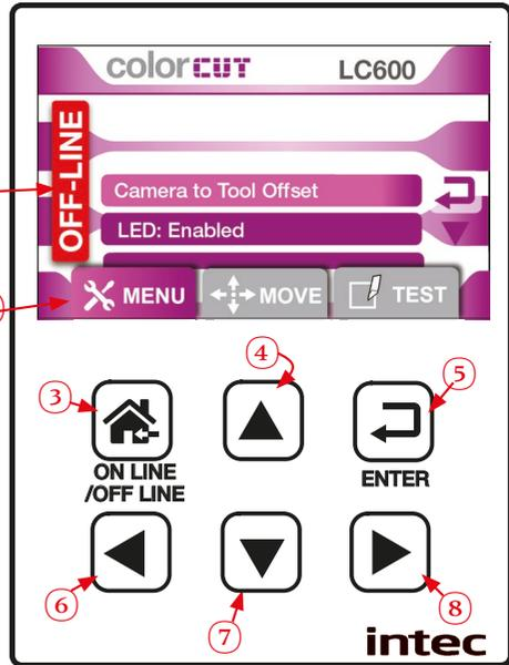
When the main 'MENU' screen is displayed, the options available will be displayed in the LCD panel screen. Press the [DOWN] DOWN arrow button 7 on the key pad to scroll down the list. Press the [UP] UP arrow button 4 on the key pad to scroll up the list.
